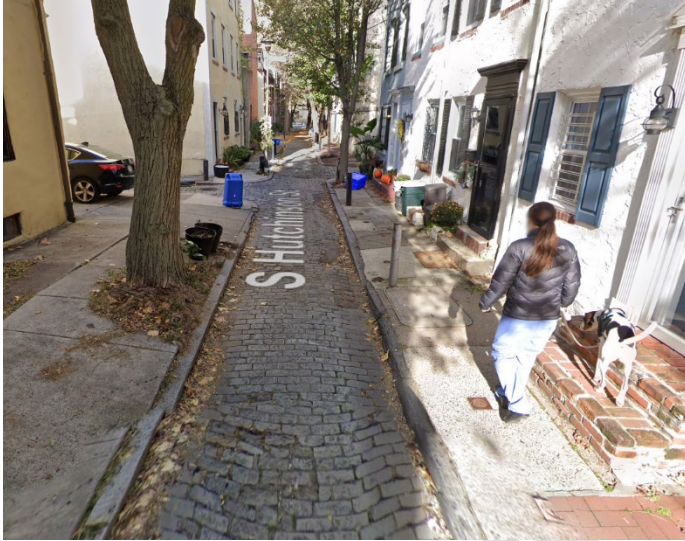
Figure 3.7: This 20' wide public right-of-way in Philadelphia has 7' paver stones in the middle with 7' concrete on either side. Credit: Google
