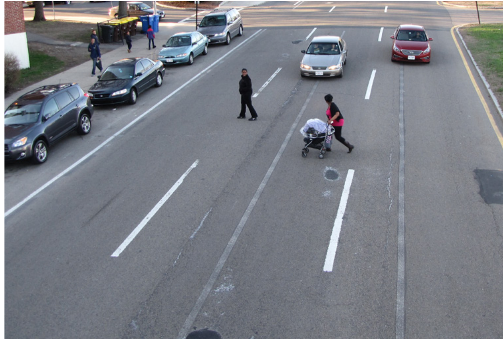
Roadways that do not have dedicated crossing areas can put pedestrians in dangerous situations when they cross the roadway.
